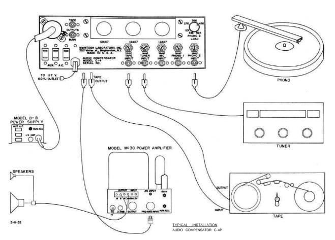
PHONO 1 Channel: This channel is equalized for use with magnetic phonograph cartridges. A level control is provided at the rear panel to allow use of cartridges with output voltage ranging from 3 MV to 70 MV. The termination of this channel is 100K which is recommended by several cartridge manufacturers. If a lower termination is desired, a resistor may be placed across the input.
